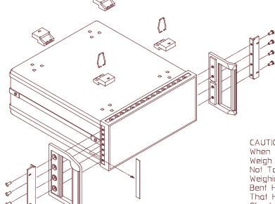
CAUTION: Use Two (2) Handles When Lifting Units That Weigh Over 18.2kg (40lbs). Not To Be Used On Units Weighing Over 36.4kg (80lbs). Bent Handles Indicate Units That Have Been Droped And Should Be Replaced.
