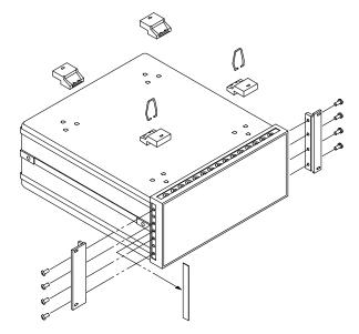
CAUTION: THIS KIT CONTAINS ONLY METRIC HARDWARE. IF INCH HARDWARE IS NEEDED ORDER INCH HARDWARE KIT #5062-4078. INSTRUMENTS WITH METRIC CABINETS HAVE THE WORD "METRIC" CAST ON TOP OF THE FRONT FRAME (UNDER THE TRIM).
