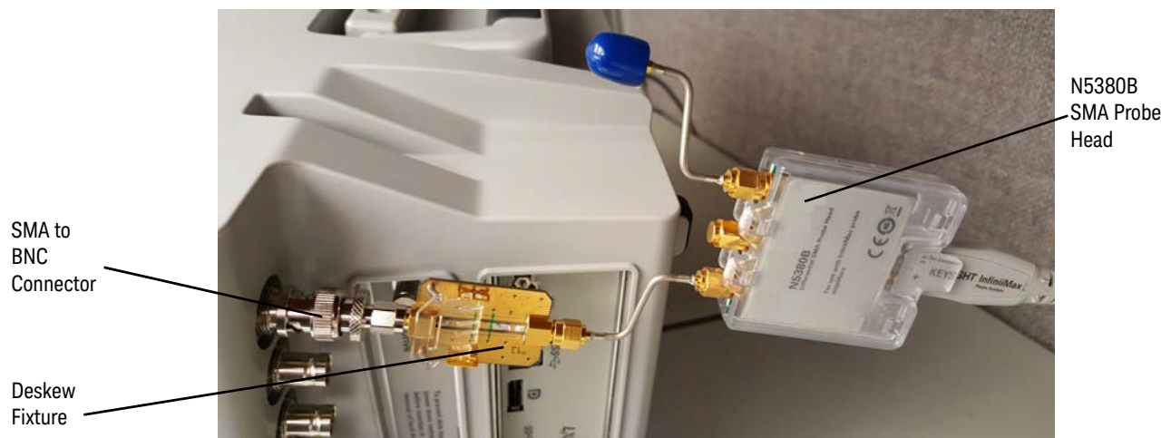
Figure 112 Connecting the SMA Probe Head and Deskew Fixture
