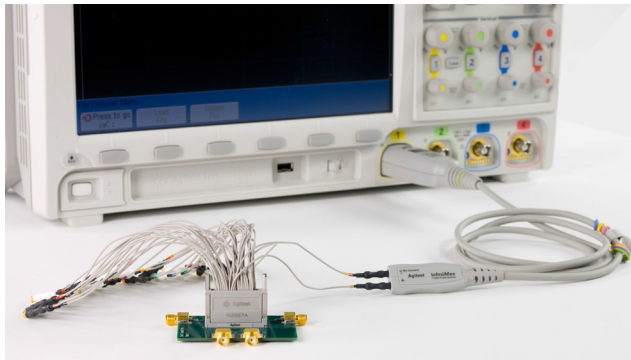
Figure 82 Soft Touch Head Connected to Probe Amplifier
