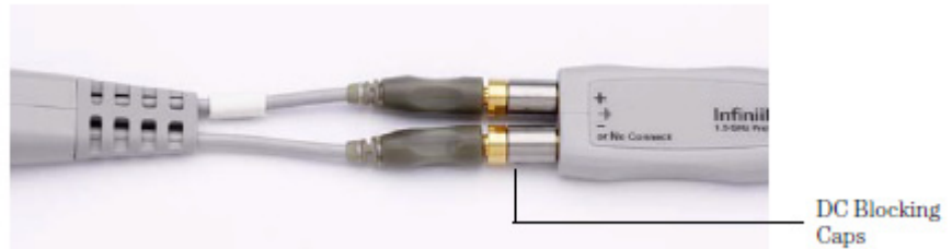
Figure 17 Blocking Caps Between Probe Amplifier and Head
