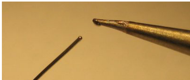
Figure 66 Small Amount of Solder Added to Soldering Iron Tip
