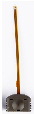
Discoloration after usage under high temperatures
