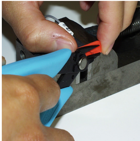
Figure 93 Cutting Wires Flush with Gauge
