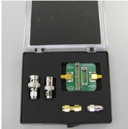
Figure 113 N2887-60002 Calibration/Deskew kit
