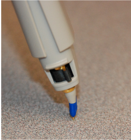
Figure 28 Proper Vertical Orientation of the Blue Tips
