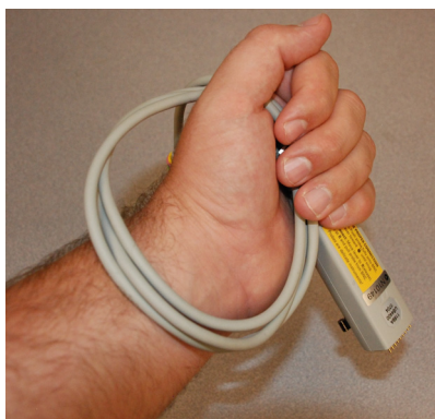
Figure 6 Recommended Coil for Storage
