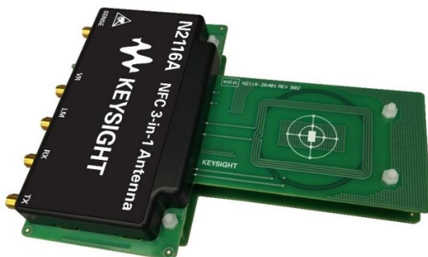
Keysight's N2116A 3-in-1 programmable NFC reference antenna.
