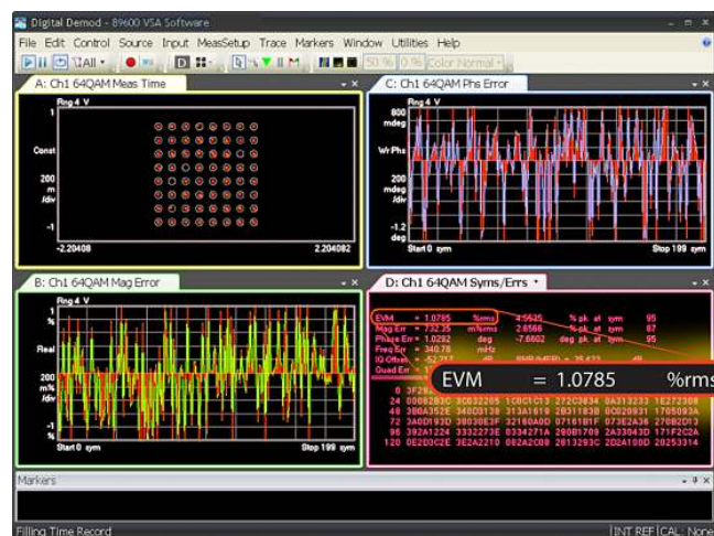
Figure 5. Constellation diagram and EVM of 64-QAM baseband signal with added noise
