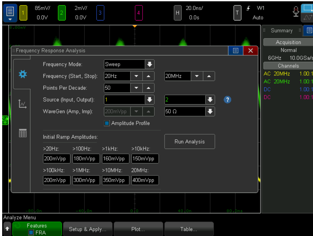
Figure 4. Optimize test signal amplitudes with Amplitude Profile.
