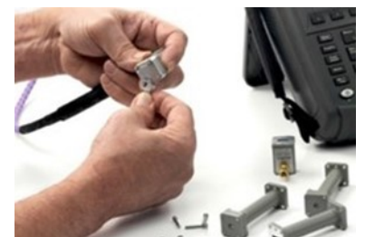
Easily use waveguides with FieldFox
