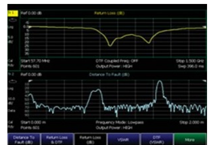
View return loss and DTF simultaneously
