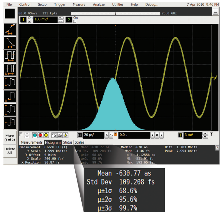
Jitter measurement floor of less than 100 fs.
