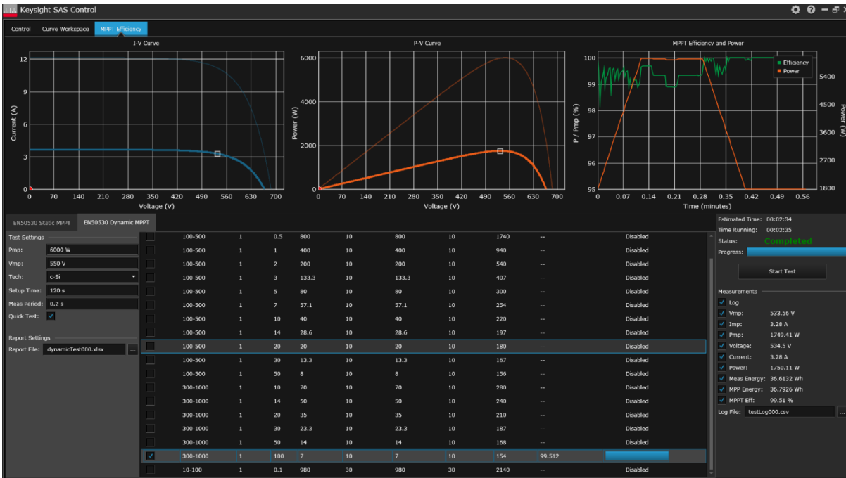
Figure 17. SAS Control Software performing dynamic EN50530 MPPT test
