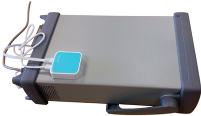
Figure 1. Shown here is a nano router on top of a 34972A with a LAN and power cables.
