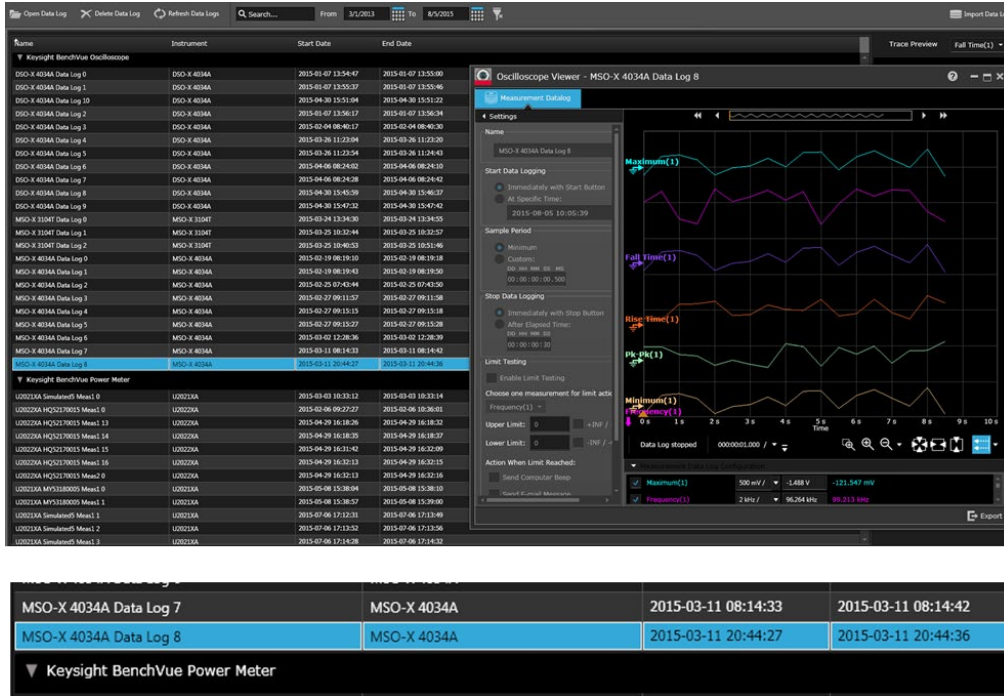
Figure 8. With BenchVue's Data Manager, data regarding a user's start and end time is logged for later reference.
