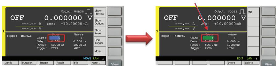
14) Or press **INF.** to set it to **INFINITY** if you'd like to continue to source pulses. If you set the trigger count to INFINITY be sure you abort the process at the end of the test.
