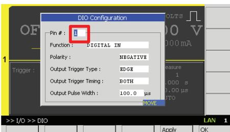
9) Press **More...** repeatedly until **Pin 9** appears in the Assist keys and then select **Pin 9** to specify the **Digital I/O pin number**, the properties of which are configured.
