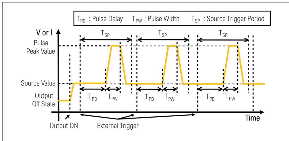
Figure 2. Timing chart for the pulsed outputs
