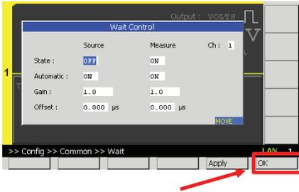
5. Initiate the channel to wait for an external trigger signal
