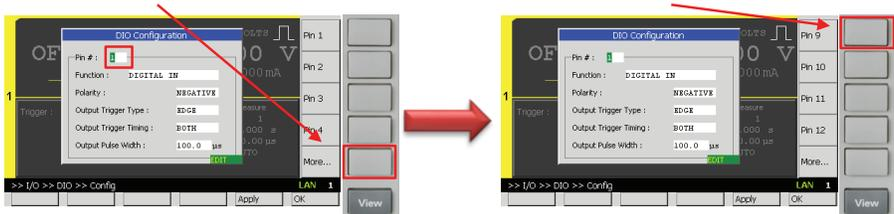
10) Rotate **Function** to select the **Input/output function** and press **Function** to edit it. Then press **TRIGGER IN** to set it to **Trigger input**
