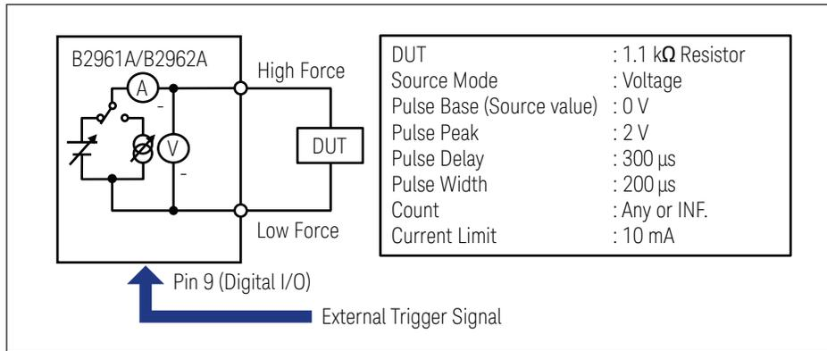
Figure 1. Connection diagram and basic condition
