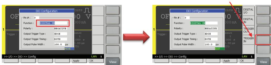
11) Rotate **Polarity** to select the **Polarity** and press **Polarity** to edit it. Then press **POS.** to set it to **Positive polarity**.
