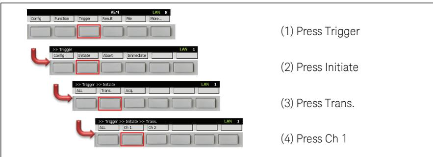
Now, the B2960A series is ready to receive an external trigger signal. Send the external trigger signal to the B2960A series to generate a pulsed signal.
