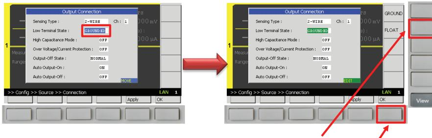
If the low terminal state of the channel is set to FLOATING, you can see the status indicator on the GUI as below, although no indicator can be seen on being set to GROUNDED.
