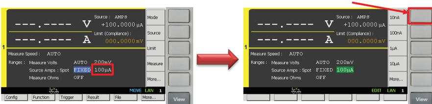
4) Press **Source** to edit the **Source value**, and then enter **0.001 nA (1 pA)** to set the **Source value** to **1 pA**.
