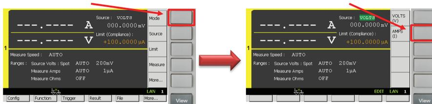
2) Rotate and press
