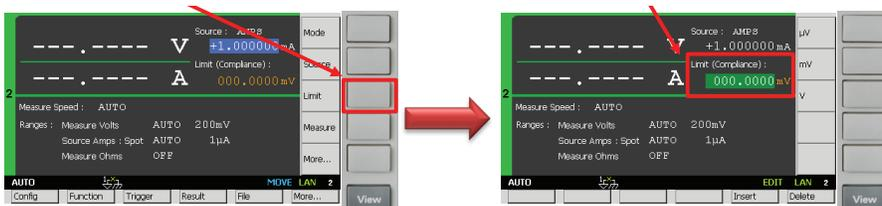
4) Press **On/Off** for the channel 2 to switch on its output terminal and enable the DUT.
