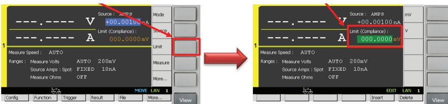
6) Press **Measure** to configure the **Measurement parameter**, and then select **VOLTS (V)** to set the **Measurement parameter** to **Voltage**.
