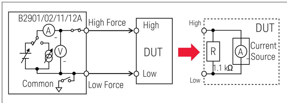
Figure 1. Connection diagram and basic condition
