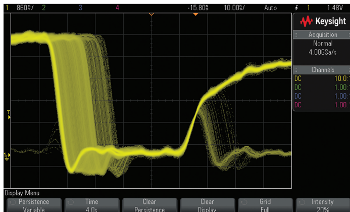
Figure 1. An update rate of 1,000,000 waveforms/sec easily captures infrequent glitches and jitter that other scopes miss.
