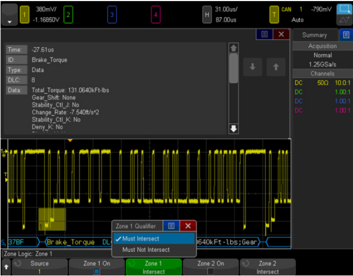
Figure 11. Characterization CAN bus arbitration using the oscilloscope's zone triggering capability.
