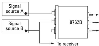
Figure 4. Multi-source switching
