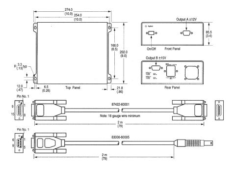
The Keysight 87422A power supply provides the dc power needed to bias the 83020A. DC cables shown above shipped with power supply. Dimensions in millimeters and (inches).
