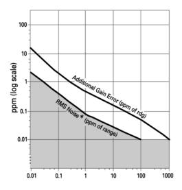
Integration time in number power line cycles (NPLC, log scale)
