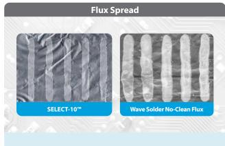
Controlled flux spray pattern for board cleanliness by SELECT-10
