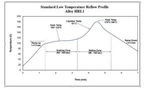
The general recommended convection reflow profile for the NP510-LT HRL1 is shown here as a starting point. Your final profile will depend on your board mass and component combination. NP510-LT HRL1 has excellent solderability and wetting capabilities in air or nitrogen reflow atmospheres reflow equipment. Your optimal profile may be different from the basic graph. Please contact Kester Technical Support if you need profiling advice.
