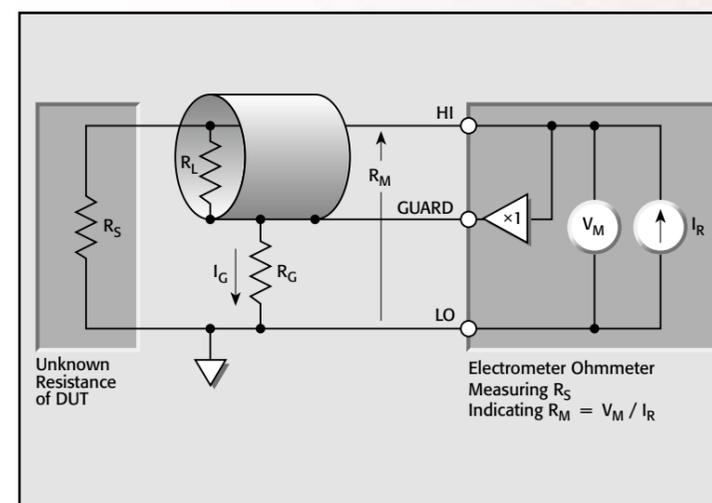
**Figure 17: Guarding Cable Shield to Eliminate Leakage Resistance**
