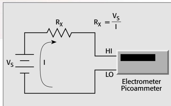
**Figure 1: High Resistance Measurement Using External Voltage Source**
