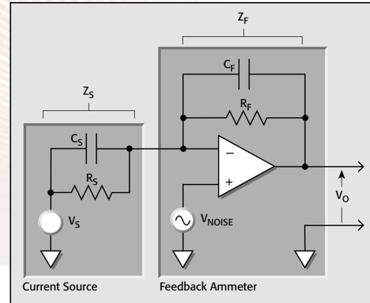
Figure 4: Simplified Model of a Feedback Ammeter
