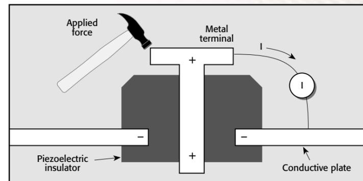
**Figure 10: Piezoelectric Effect**
