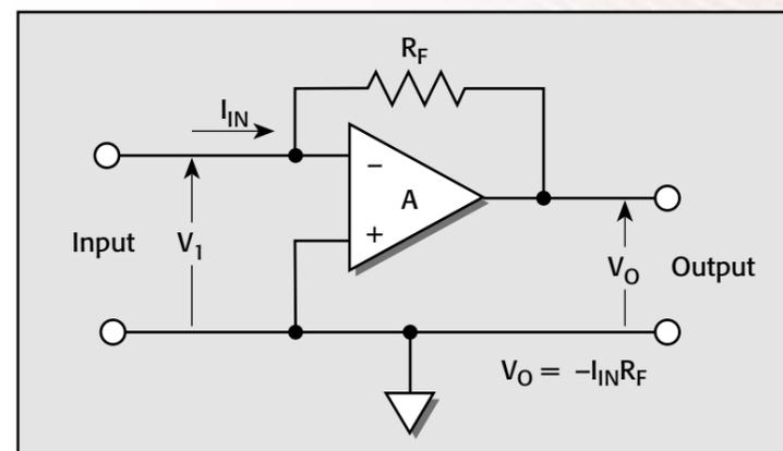
**Figure 3: Feedback Ammeter**
