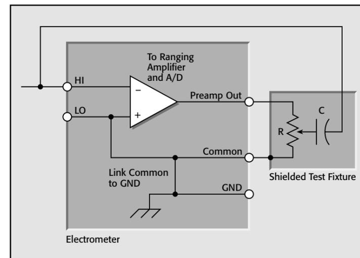
**Figure 12: External Damping Circuit**
