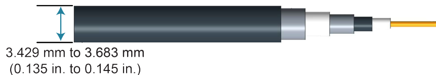
Figure 5: SC-22 triaxial cable dimensions
