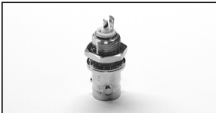
CS-630: 3-lug female triax bulkhead connector for soldered connection. Mates with CS-631. For use with: Fixtures, 6487, 6517A, 6517B
