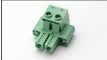
CS-1592-2: 2-pin male screw terminal connector plug. Rated 50A. Mates with the Model CS-1626-2 screw terminal block.
