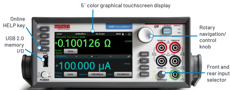
2450 front panel with high-resolution, capacitive touchscreen.
