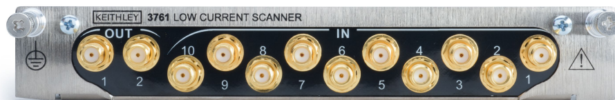
Figure 2: Model 3761 card connectors
