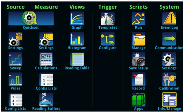
The graphical SMU's icon-based menu structure helps even novice users configure tests quickly and confidently.
