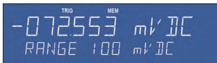
Figure 1. Storing readings to the data buffer.
