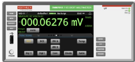
The DMM7512 virtual front panel displays a conventional DMM front panel.
