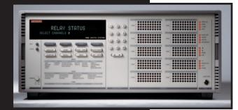
The Model 7002 Switch System is a 10-slot mainframe that supports up to 400 2-pole multiplexer channels or 400 matrix crosspoints. The front panel includes a unique interactive display of channel status for quick programming. Scanning speeds of up to 300 channels per second are possible with the high density switch cards. The wide selection of more than 30 different switch cards makes the 7002 one of the most flexible switching mainframes available.
