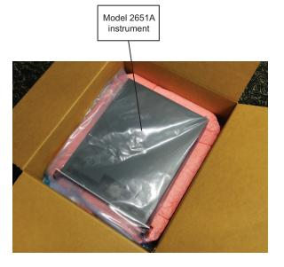
6. Inspect the instrument for any obvious signs of physical damage. Report any damage to the shipping agent immediately.
