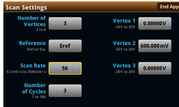
2450-EC Cyclic Voltammetry Test Configuration Screen
