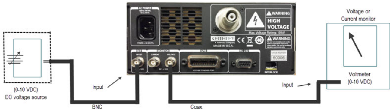
Figure 6: Model 2290-10 analog input control and voltage or current monitor connections
