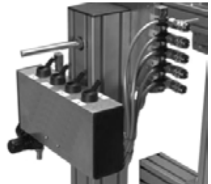
Pneumatic controls to test the functionality of the custom EOAT fixture.
