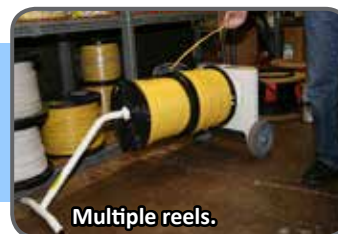
Feed the spool rod through the reel's ID and use the spool rod as a mechanical advantage for lifting the cable reel in upright position.
