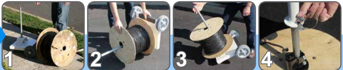
Feed the spool rod through the reel's ID and use the spool rod as a mechanical advantage for lifting the cable reel in upright position.
