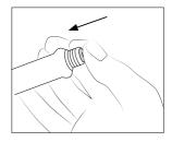
Gently push the Seal inside the handle until it is completely into the Handle. Handle and Seal edges have to be aligned.
