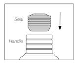
Note the Seal mounting position. The chamfered side has to be positioned towards the Handle.
