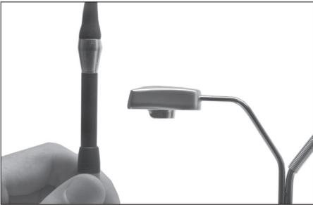
When the tool is lifted from the holder the tip will heat up to the selected temperature.
