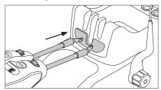
Press the cartridges against the extractor and make sure that the cartridge are inserted up to the mark\*.
