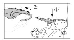
Place the cartridges in the extractor (1) and pull the tweezers to remove them (2).
