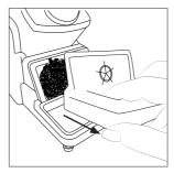
Remove the wiper by pulling it out.
