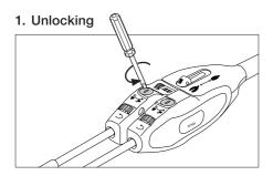
Unlock the fixing screws.
