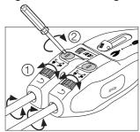
Slightly turn the wheels to align the cartridges as required (1). Then lock the catridge fixing screws\* (2).
