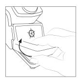
Lift the wiper at its front edge.
