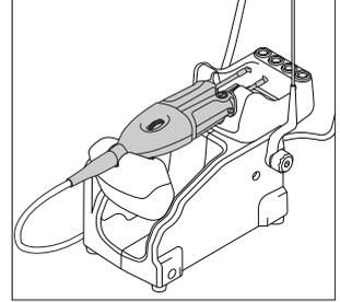
After longer periods of inactivity, the power is cut off and the cartridges cool down to room temperature.
