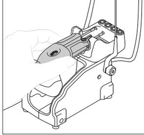
When the wire stripper is in the stand, the power falls after a specified time.
