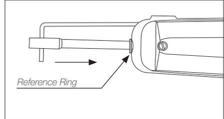
Insert the cartridge until the reference ring touches the wire stripper. Take the ring as a reference and check that both tips match.
