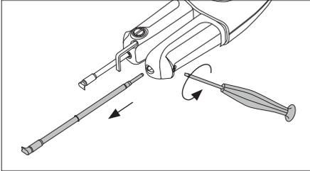
Loosen the screws and remove the cartridges.
