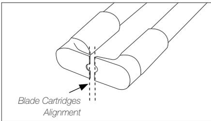
Align the tip edges and fix the cartridge in its working position.
