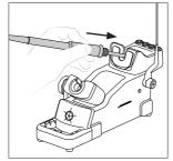
Place the handle on top of the new cartridge and press the handle down.
