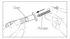
Insert the plunger into te seal and press the seal against the solder paste to eliminate the air inside the barrel.
