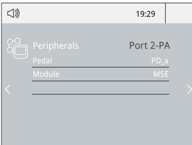
2. Select the pedal from the list (*Note that your first connection is denoted as "a", the second being "b", etc. (e.g. PD\_a, PD\_b,...).*)
