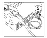
Plug in the pedal connector (5) to the equipotencial connector at the back side of the station.
