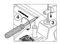
Reassemble the tool holder (3) and fasten the locking screw with the allen key (1).
