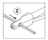
Insert the tool holder (2) by its bottom side through the connection.
