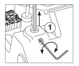
Disassemble the tool holder from the station with a 1,5mm allen key (1).
