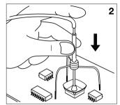
To desolder small components you must use the protector + tripod as shown in drawings 1 and 2.
