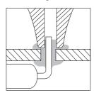
When the solder liquefies, gently rotate the tip so that the component terminal can be lifted off.
