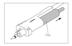
**3.** Insert a new filter (ref. 0008473) into the tool and mount the tube onto the filter.
