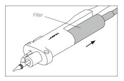
3. Use the cleaning brush (ref. 0008297) to clean the solder collector inside or replace it for a new one.
