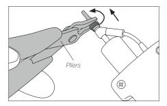
2. To fasten the tip, do not hold it on the spring clamp. Place the pliers directly in front of the spring.
