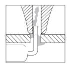
Press the vacuum pump button long enough to remove the solder.
