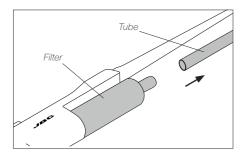
2. Remove the filter form the tool.
