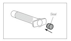
Take the barrel filled with solder paste and place the corresponding seal into the barrel.
