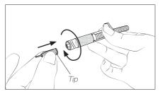
Thread the tip onto the syringe barrel.
