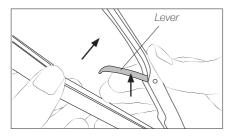
Open the DPM by lifting its upper part and the lever.
