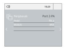
2. Select the pedal from the list (Note that your first connection is denoted as "a", the second being "b", etc. (e.g. PD\_a, PD\_b,...).
