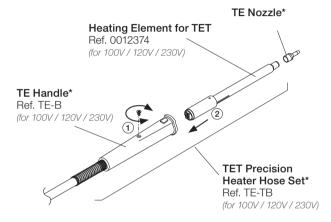
**Note:** Only perform this operation when the heating element is cold and the unit is disconnected from the mains.
