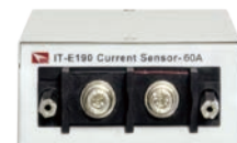
IT-E190-60A (option) Current sensor Applicable models: IT9100, IT9500
