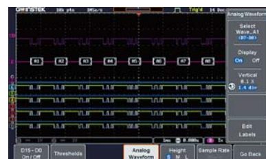
Display analog waveform converted from digital signal
