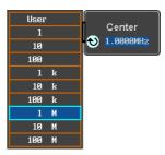
4. Alternatively, select *User* from the list of frequency or press the *Select* key. Use the arrows to select a base unit and the variable knob to further tune the selected base unit.
