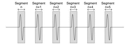
As shown above, the memory is divided into segments to increase the number of events that can be effectively captured with the same acquisition memory. Also notice that the scope doesn't need to rearm the trigger between each segment, this makes the segmented memory function especially useful for high speed signals. The time between each segment is also recorded so that accurate signal timing can also be measured.
