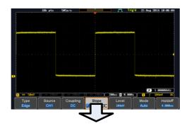
11. Press the relevant function key again to reduce the bottom menu. For example: press the Trigger Menu key to reduce the trigger menu.
