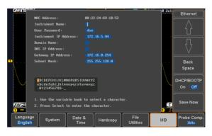
6. Use the *Up* and *Down* arrows on the side menu to navigate to each Ethernet configuration item.
