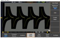
10. Press the *Auto Mask* button from the bottom menu to close auto mask function.
