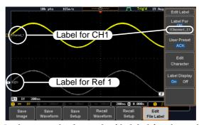
In the example above, the file label for channel 1 is displayed next to the channel indicator and is also displayed in the *Edit Label* menu. The Ref\_1 file label is shown next to the reference indicator.
